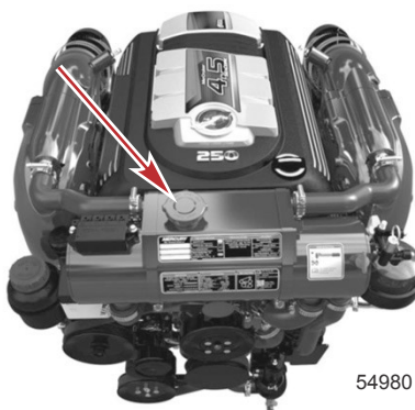
Heat exchanger cap
