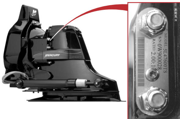
Bravo sterndrive information on ground plate
