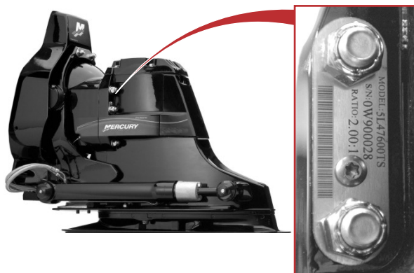
Bravo sterndrive information on ground plate
