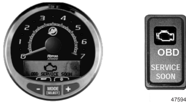
SC 1000 gauge and service engine light
