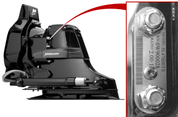
Bravo sterndrive information on ground plate
